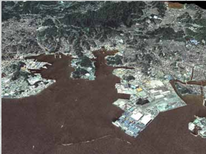
3D Visualization of Textured DSM (overlaid with 2.8 m Multispectral Image)
