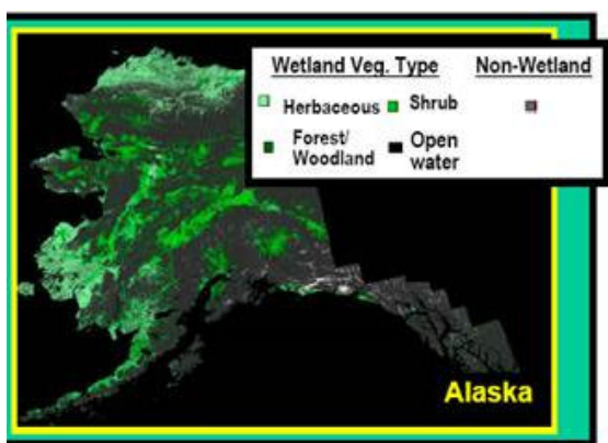
Figure 2. Wetlands map of Alaska derived from L-band JERS SAR backscatter imagery. The 1990's-era JERS data set constitutes a pathfinder for application of satellite-borne SAR for mapping global wetlands. (Whitcomb et al., 2009).
