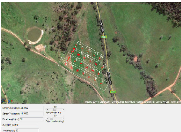
Figure 2. Flight planning software. Flight grid is approximately 200 x 100 m which represents a single flight sequence (5 mins flight duration)
