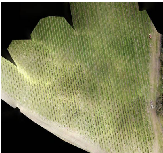
Figure 6. Example ortho-mosaic of visible vineyard imagery made up from 48 images. Area is approximately 200x150m
