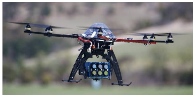
Figure 1. Oktokopter fitted with multispectral camera.
