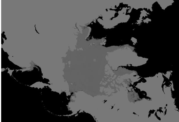
Figure 1. AMSR-E northern hemisphere sea ice concentration from December 19, 2010. Valid data, missing data and land are all represented in the 1-byte integer.
