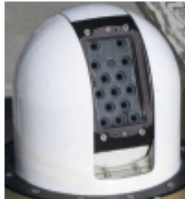
Figure 2. AATS-14—Ames Airborne Tracking Sunphotometer will make simultaneous measurements for empirical characterization of the atmospheric column.
