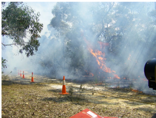
Figure 4: the spectrometer's telescope is in the foreground to the right and the retro reflectors are just visible at the end of the line of traffic cones at the Gibberagong hazard reduction burn.
