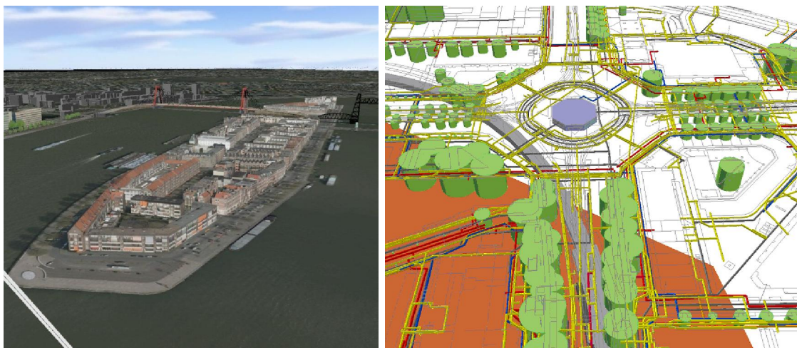
Fig 1: City of Rotterdam: 3D city model (left) and b) 3D underground infrastructure (right)
