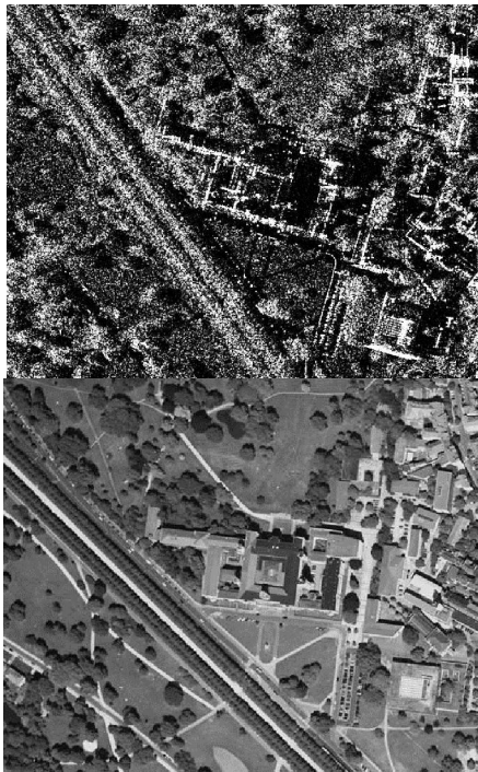
Figure 8: TerraSAR-X radar spot light image with 1m GSD
