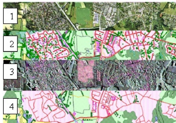
Figure 9: above: optical image, followed by mapping with optical image, below: SAR image followed by mapping with SAR image (Lohmann et al 2004)
