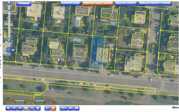
Fig 5. Information about a parcel and Cadastre vector data imaged with aerial orthophoto mosaic
