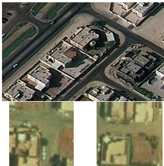
Figure 12: above GeoEye-1 image with 0.5m GSD, below samples from aerial photos with 0.7m GSD
