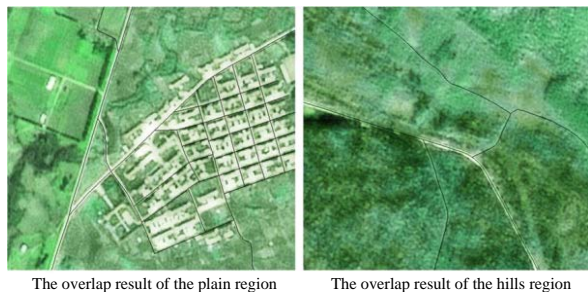
Figure 4. The result of overlap between GCP Image Chip and the 1:10,000 DLG
