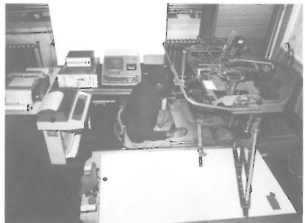
Fig.5 Galileo Stereosimplex IIC with Wang 2200 Desk-Top Computer for computer-assisted stereoplotting.
