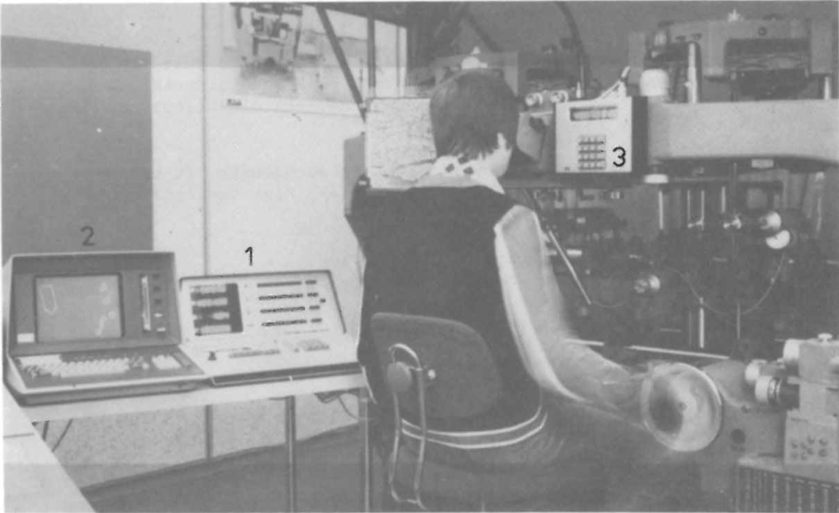
Figure 2. Photogrammetric digital mapping. (1) Registration unit. (2) Desktop computer. (3) Keyboard.
