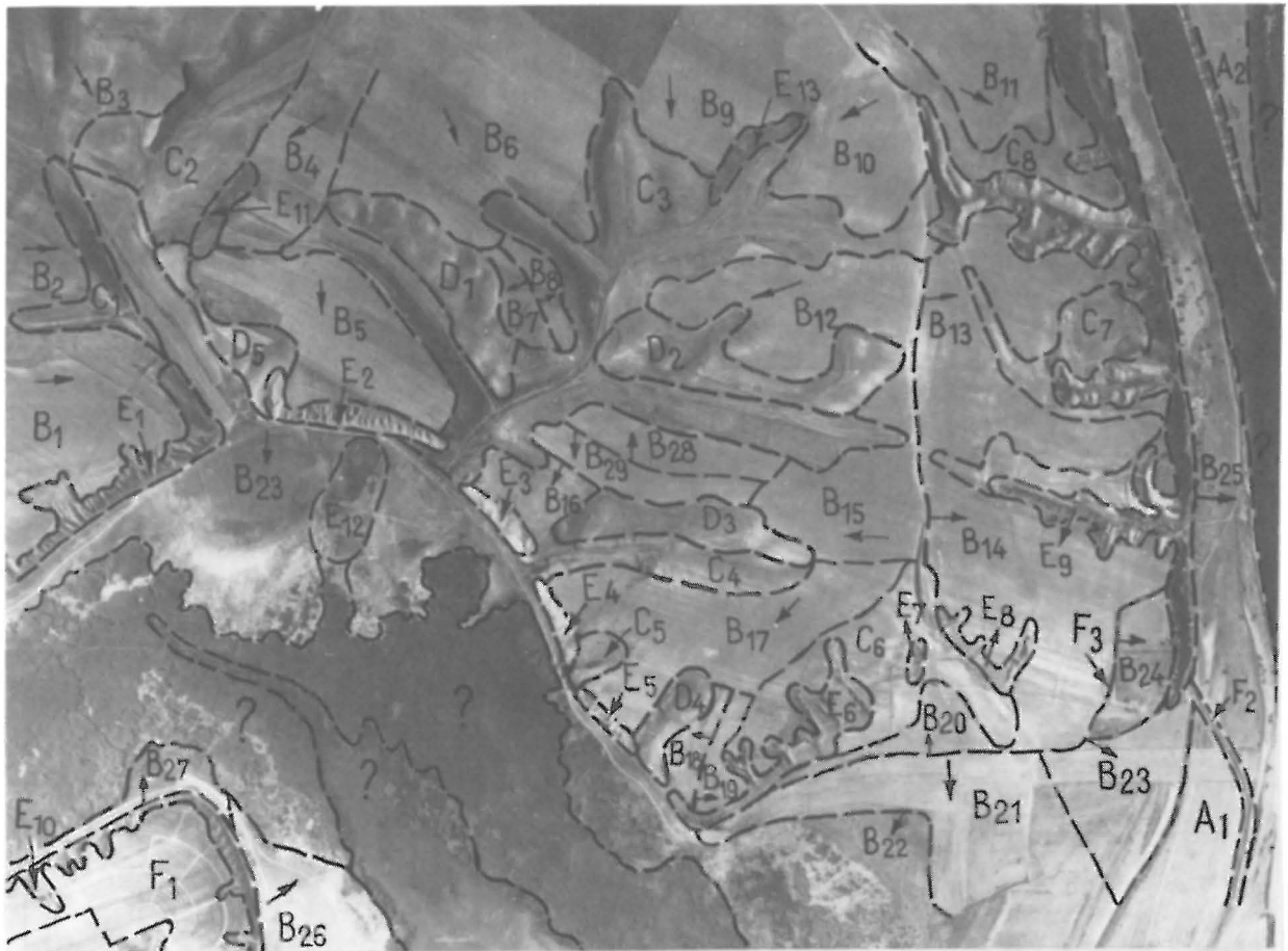
Fig. 3. Delimitation of the terrain configurations or accidents (area in the south-west of Dobrudja, on the right bank of the Danube River). A - horizontal zones ; B - sloping flat areas ; C - gently rolled areas ; D - powerfully rolled areas ; E - natural terrain "accidents" ; F - artificial terrain "accidents"
