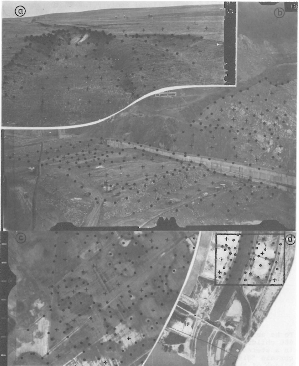
Fig.5 The selection of characteristic points defining the forms of relief and the natural or artificial "accidents" a.-ravine within the hydrographic basin of the Buzău River (terrestrial photograph); b.-area with hollows situated north of Bucharest (aerial photograph); c.-portion of the zone of the Siriu dam during the excavations (terrestrial photograph); d.-portion of the headwater channel for the „Carasu” irrigation system.
