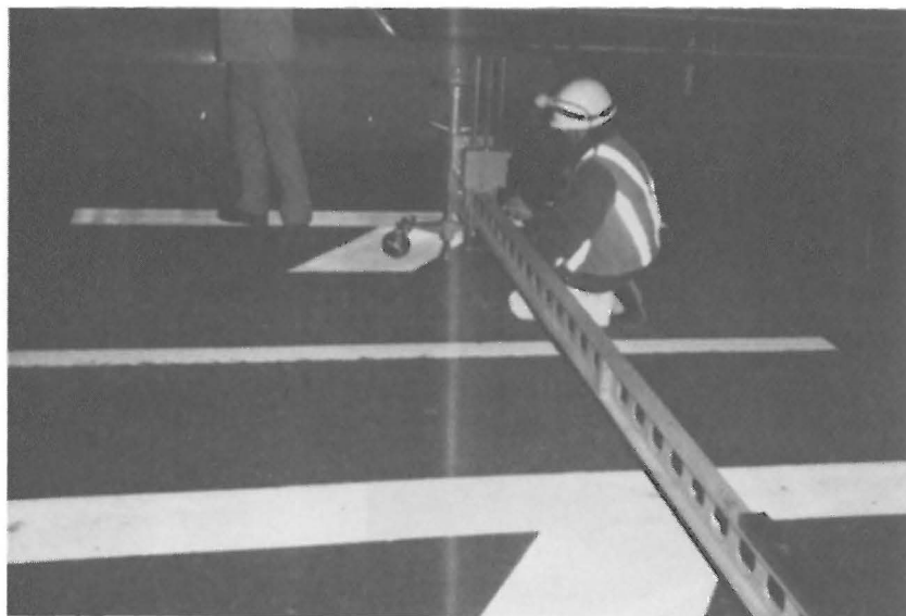
Figure 2 Surveying using a profilemeter
