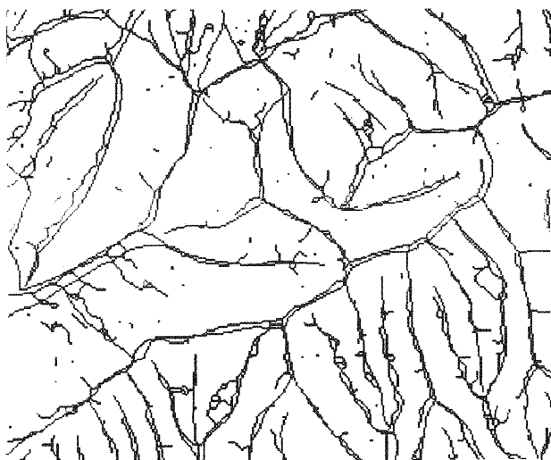
Fig. 10: Superimposition of skeletons from manual and automatic extraction (the 'fringes' belong to the automatic one)
