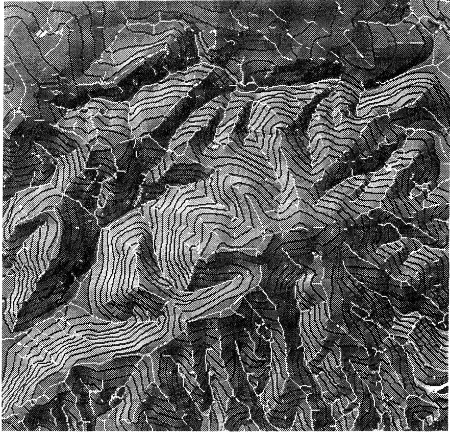
Fig. A2: Extracted skeleton lines and contours
