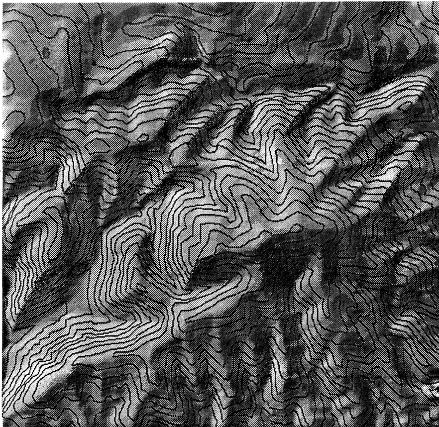
Fig. A3: DTM from contours and skeleton
