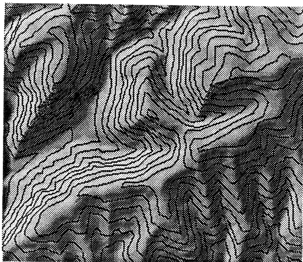
Fig. 9: DTM from contours and skeleton
