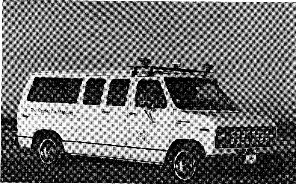
Plate 1: Mapping Van of the Project Application of the Global Positioning System for Transportation Planning
