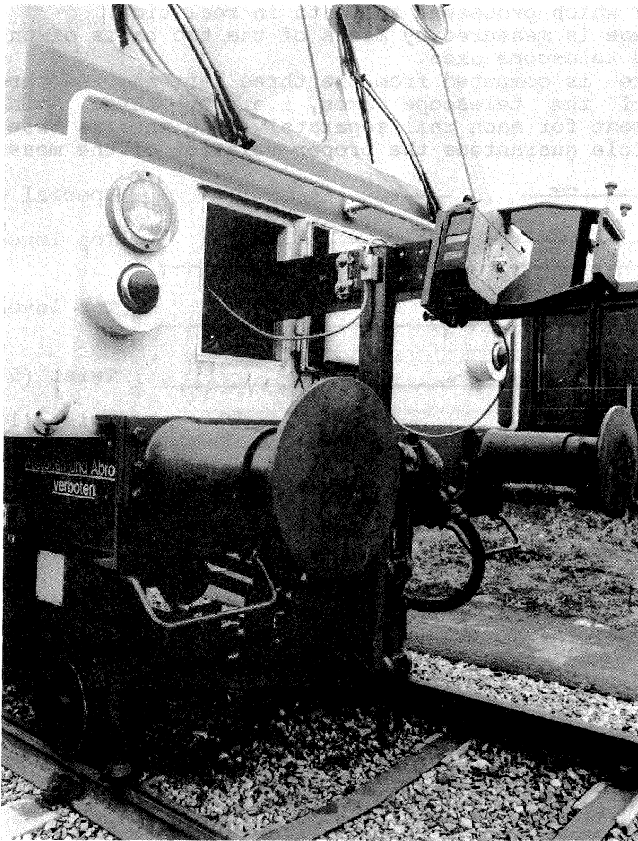
Fig. 3: The impulse laser system RIEGL DM 900 in cross profile working position
