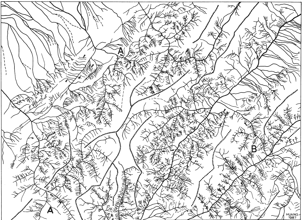
Fig. 4 Interpreted drainage map on the base of a satellite image (Fig.2). Arrows indicate faults or inferred faults.
