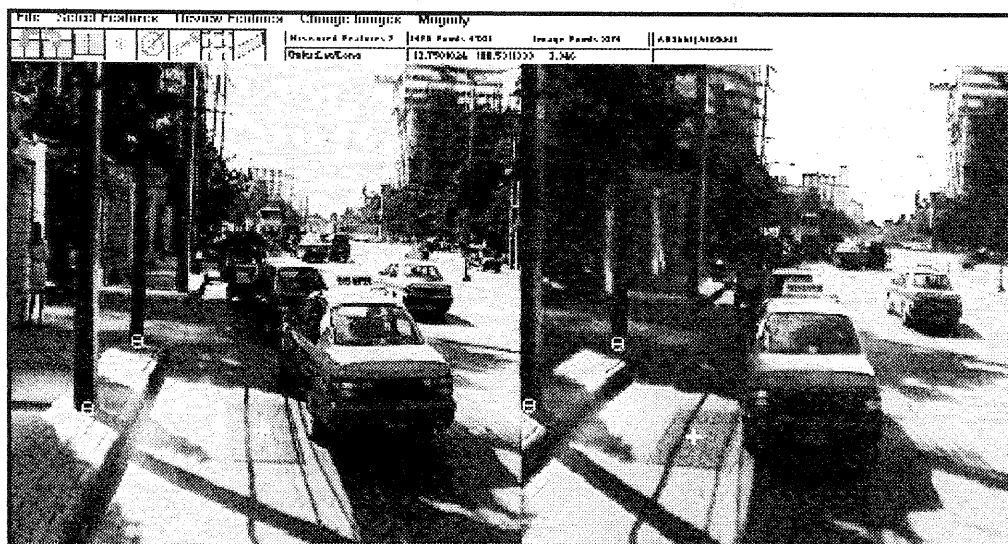
Fig. 4 Georeferenced stereo image pair taken from Bangkok, Thailand. Two poles and one manhole are extracted from this image pair.
