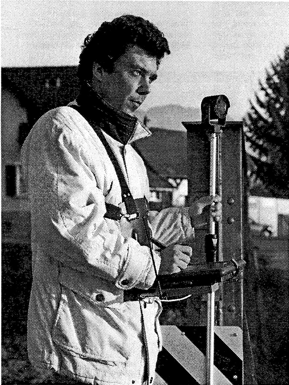
Fig. 2. Chest mounted frame for penpad. Telemetry link mounted underneath.
