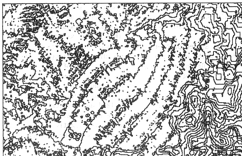
Fig.5: Contour line expression of DTM
