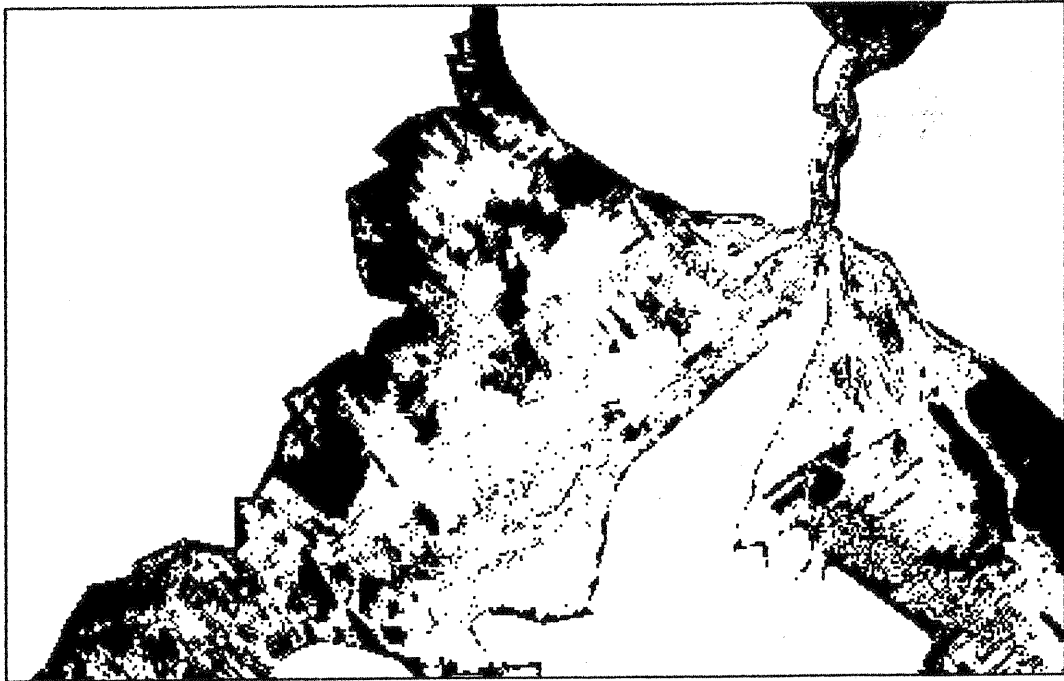
Fig. (3) - Unsupervised classified image of Landsat TM data (bands 2, 4, 7) of Talaat El-Badan area
