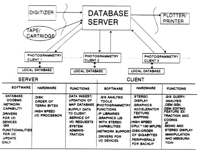
Figure 1. System Configuration and Specifications
