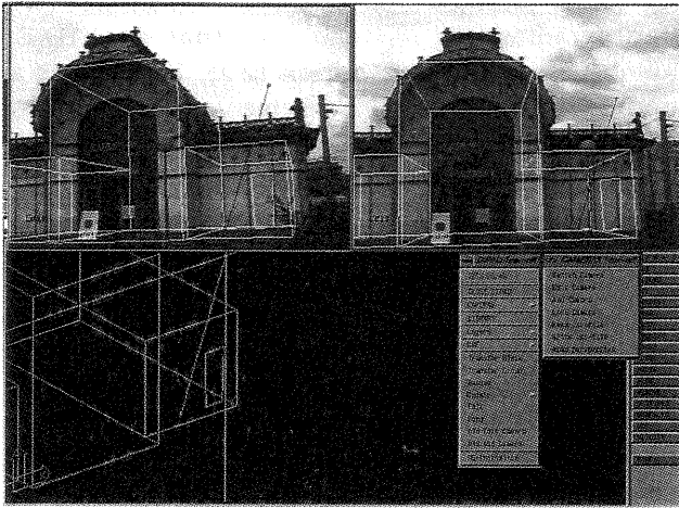
Figure 3: Using the transfer protocol the modelling in the CAAD program can be monitored in the DIPS. So the modelling of approximations is very convenient.
