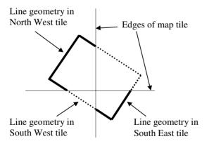
The traditional tile-based system splits features up at tile edges.
