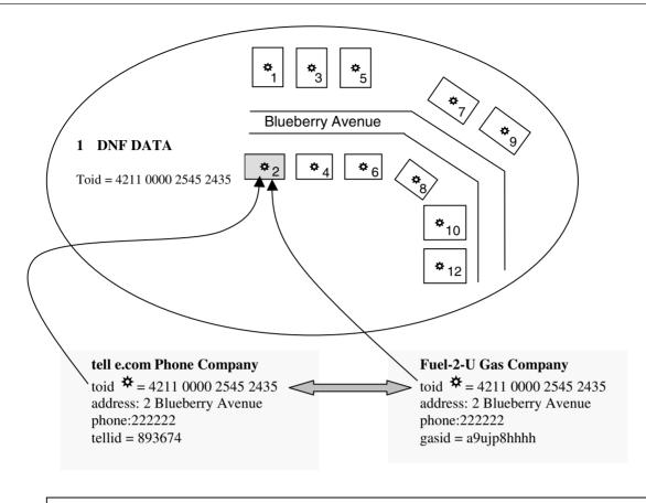
Figure 1: Many users can reference the same feature using the Topographic Object Identifier (TOID). They will be able to access change information from DNF on each feature they hold. They can also unambiguously share information about features they hold in common.
