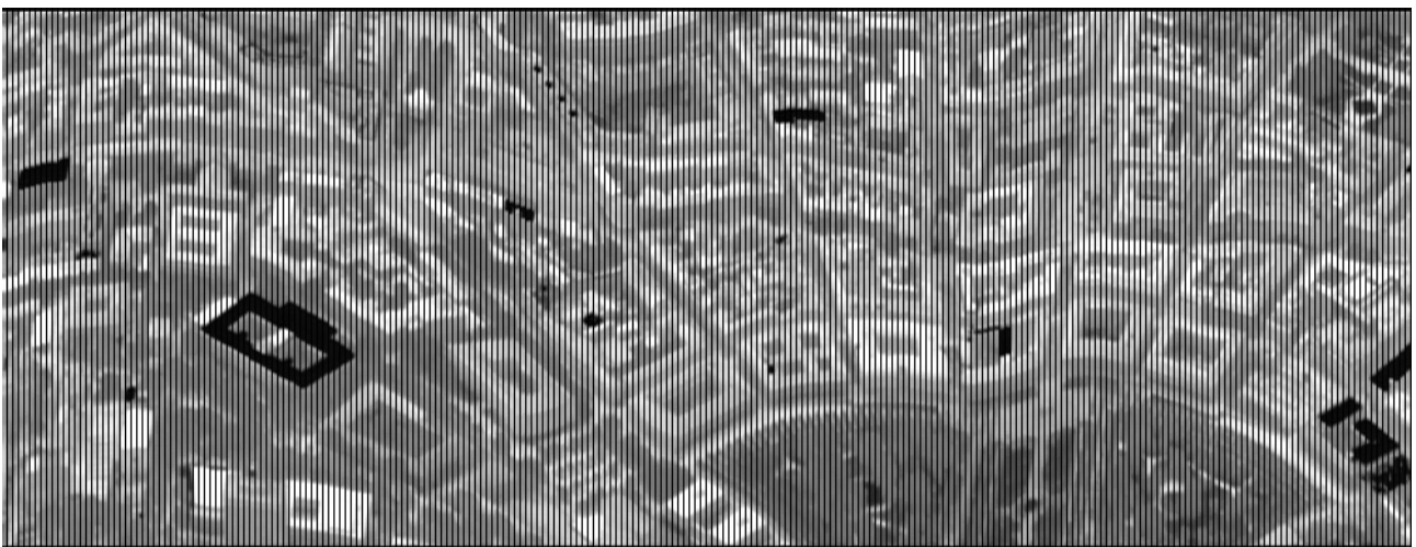
Fig. 3: Mosaicing of an infrared image sequence containing 250 frames with geometric distortions.
