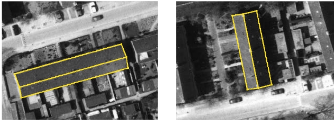
Figure 10. Reconstructed gable roof buildings projected back into the image
