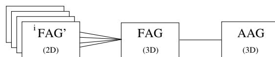
Figure 3: Relationship of the graphs {}^iFAG' of the images i , the 3D FAG and the graphs of the 3D aggregates, AAG. Some of these 2D features induce a set of 3D features and their neighborhood relationship, contained in the 3D FAG. Aggregating these features leads to entities like n -corners C^n , which in turn is part of the 3D AAG.
