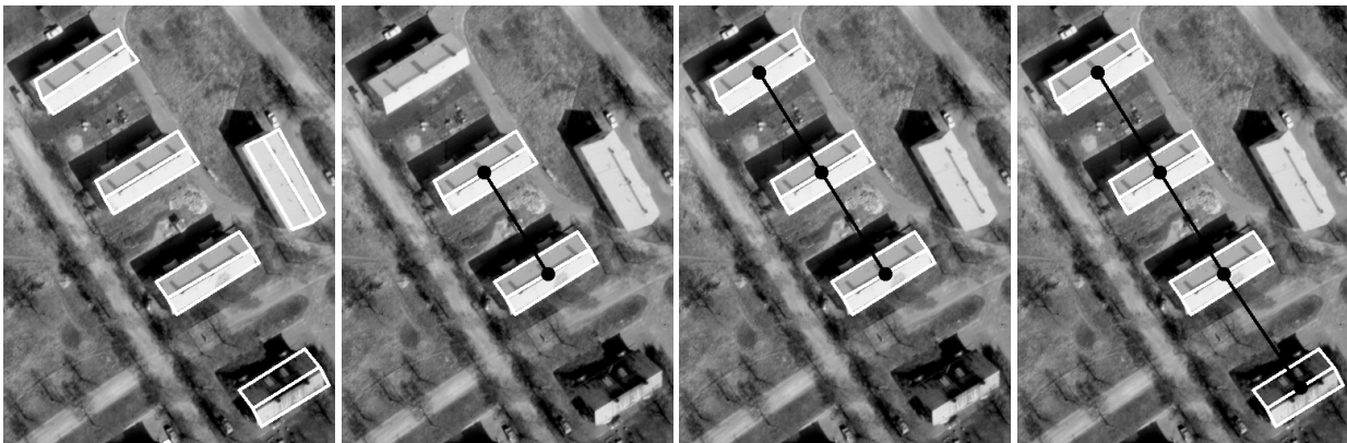
Fig. 1: Grouping a 3D-House-Row using the relations similarity and linear continuation. (3D-House-Instances generated from FLAT stereo benchmark)
