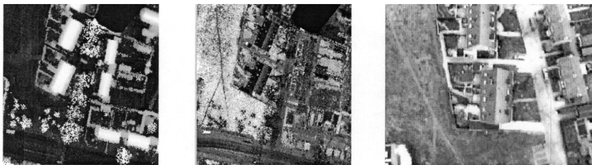
Fig. 1: Part of FLI-MAP data set; left: height image 0.5 meter grid resolution; center: reflectance image; right: video shot (not georeferenced).
