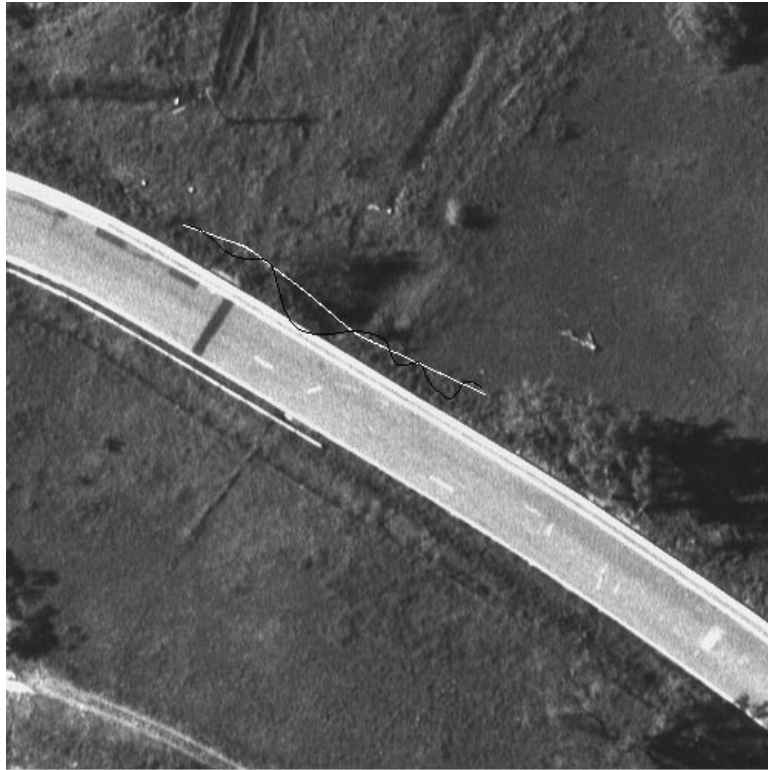
Figure 3: Feature Extraction Using Snake after 50 Iterations for Initial Configuration 2
