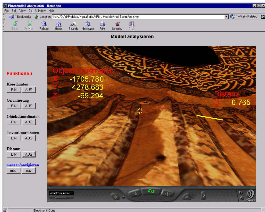
Figure 7. Detail of the dome showing a modeled structural fissure (also visible in Figure 4) and the measured coordinates at the cursor position as well as a measured distance marked at the bright line.
