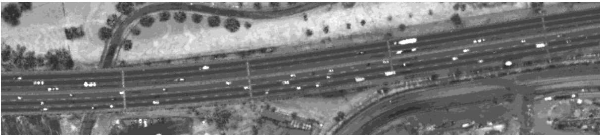
Figure 2. LiDAR intensity data of a freeway in Toronto downtown.
