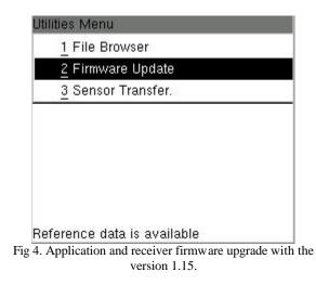
Firmware updates can only be executed from the compact flash card in the GS20: the files transfer has required more than two hours. The receiver has lost the informations of its initial configuration: it has been necessary to restart the initialization to allow the receiver to adjourn satellites configuration.
