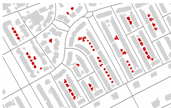
Figure 4: Segments in a part of the DSM that were classified as buildings. In red the building objects that were labelled as shed.
