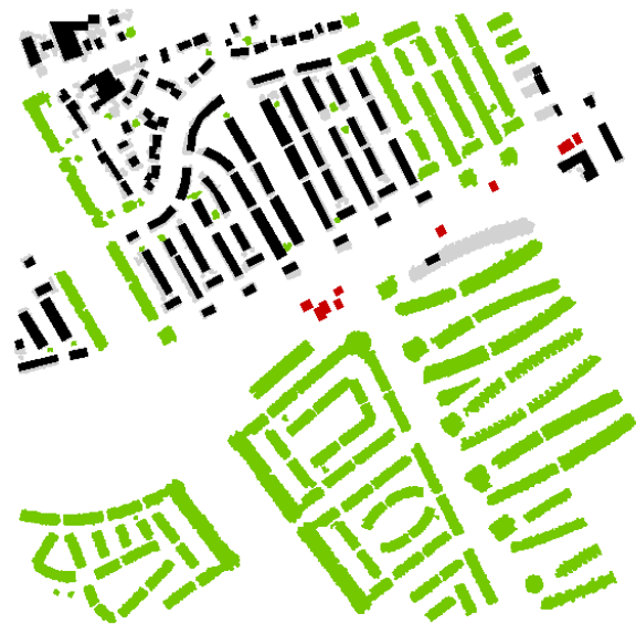
Figure 6: Results of detection of new and demolished buildings. The segments extracted from the laser data are shown in light grey and green. The map objects of the TOP10vector map are overlaid in black and red. The red objects are classified as demolished buildings. The green segments are classified as new buildings.
