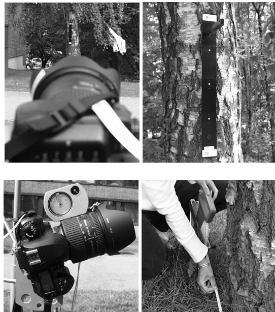
Figure 1. Image capture. Camera was rotated in the position where trunk was in the middle of the image (up left). Reference scale bar was attached to tree trunk (up right). Camera was rotated 20^\circ (bottom left). Distance to the tree was measured (bottom right.)
