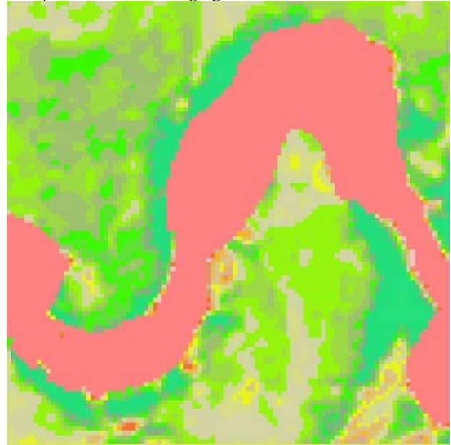
Figure 5. area 1: Differences in height between DTM based on digitized contours and DSM for area 1. Red to yellow = DTM higher than DSM. Green = DTM lower than DSM.
