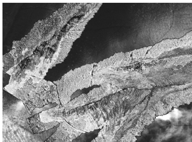
Figure 10. Particular of an orthoimage and overlay with the intensity laser data over a landslide detachment surface
