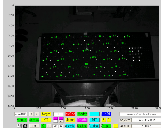
Figure 2. Model a slope displayed on a screen of the measurement system "SUBARU"
