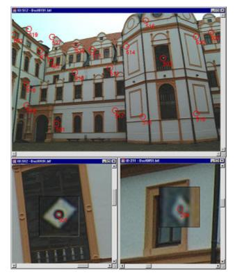
**Fig. 4:** Image point measurements of tie points (upper) and control points (lower) in one image of Celle castle
