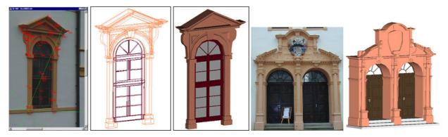
Fig. 6: Measurement, reconstruction and rendering of a window of Celle castle (from left to right), ornate doorway as a photo and as a generalized reconstructed doorway (right)
