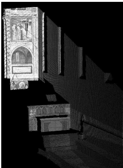
Figure 10. Effect of laser beam tilting in Optech scans
