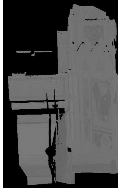
Figure 11. Intensity response of Cyrax 2500
