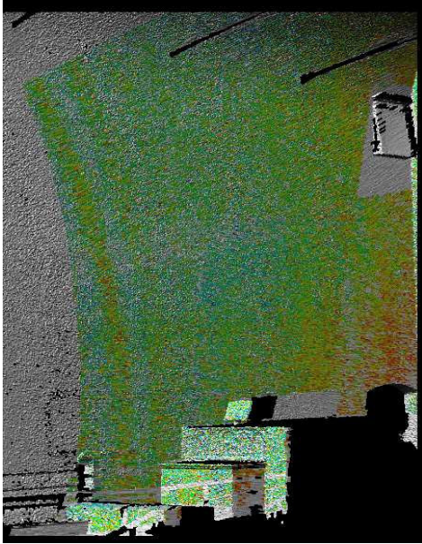
Figure 9. Errormap btw.adjacent Optech scans
