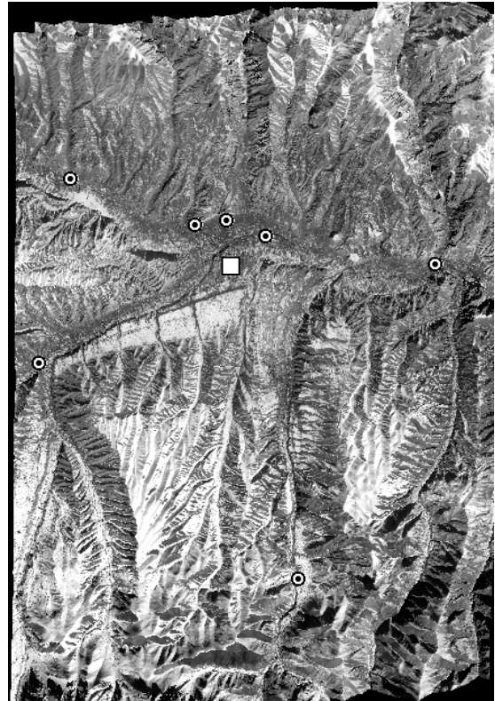
Figure 4: The distribution of the GPS ground control points on the IKONOS image mosaic. In the centre the master station position.
