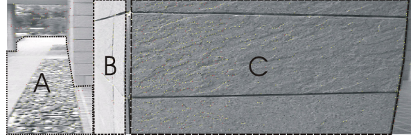
Figure 8. A test image of 3D objects, where three sets of registration parameters are used for the areas A, B, and C, respectively
