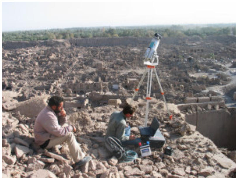
Figure 2: RIEGL LMS Z420i in Bam Citadel
