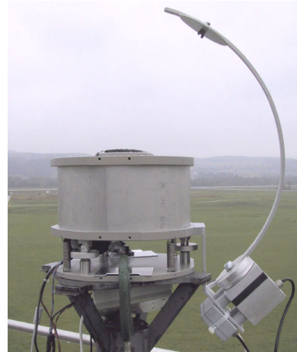
Figure 2. Ground-based imager system (Skycam).
