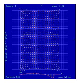
Fig. 9: Image residuals without additional parameters
