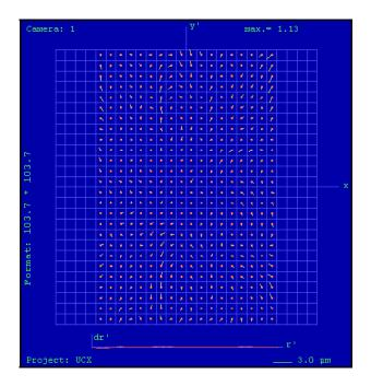
Fig. 10: Image residuals using radial distortion parameters
