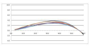
Fig 11: Radial symmetric distortion derived from various UltraCamX test flights.
