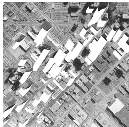
Figure 8. The result of shadow detection based on DBM
