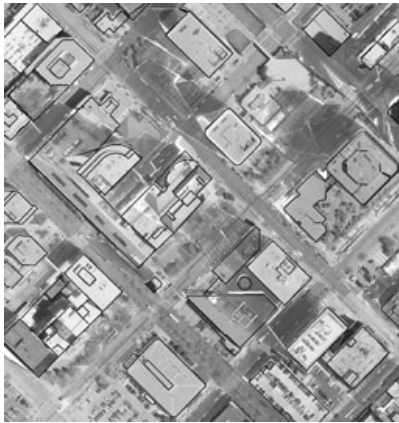
Figure 10. True orthophoto after occlusion refilling and shadow removal
