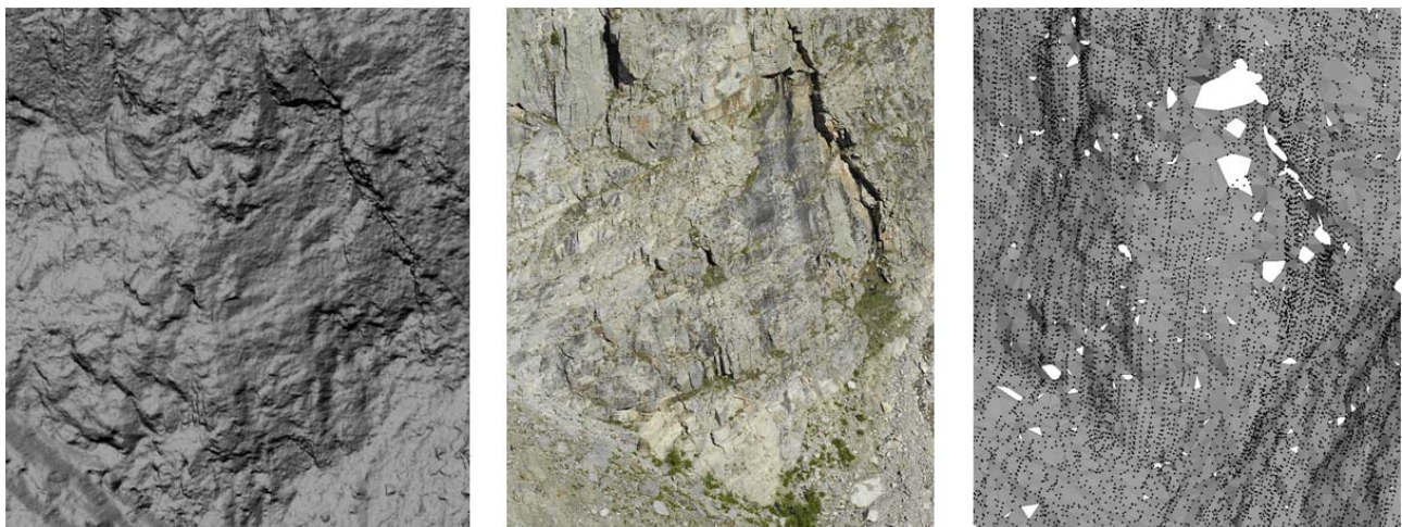
Figure 6: Left: Derived surface model from image matching, Middle: Zoom-in of an UAV-image, Right: Point cloud of Helicopter-based LiDAR projected on the derived surface model.
