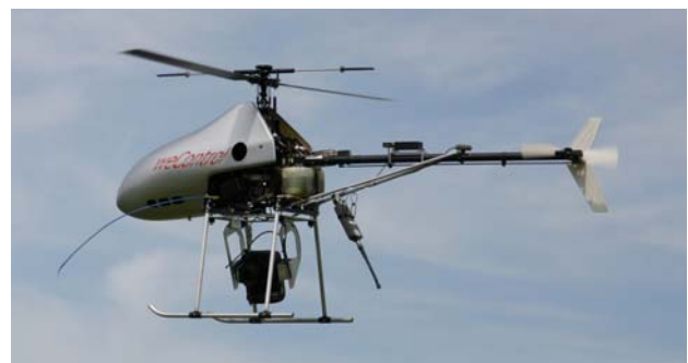
Figure 4: Our model helicopter during a test flight with the inclined camera looking perpendicular to the flight direction.
