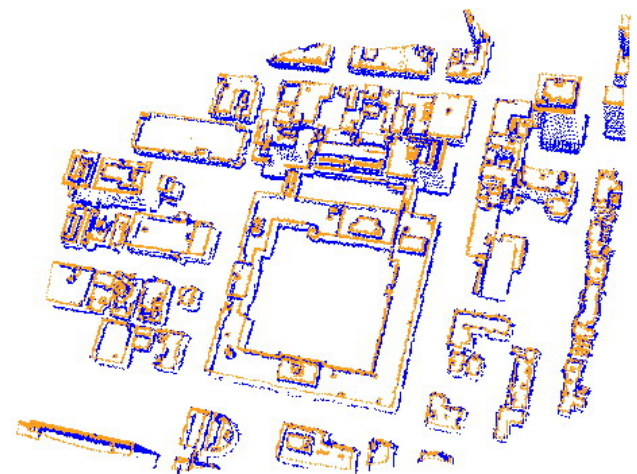
Figure 6. Edge points detected from LIDAR data. The orange denotes the edge points inside roof patches, and the blue denotes the edge points outside roof patches.
