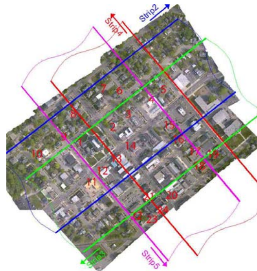
Figure 2: Highlighted buildings distributed in the area and LiDAR strips' orientation
