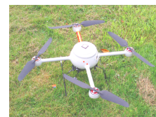
Figure 1: Used hardware. Drone MD 4-200 from Microdrones © equipped with a Panasonic Lumix video camera
